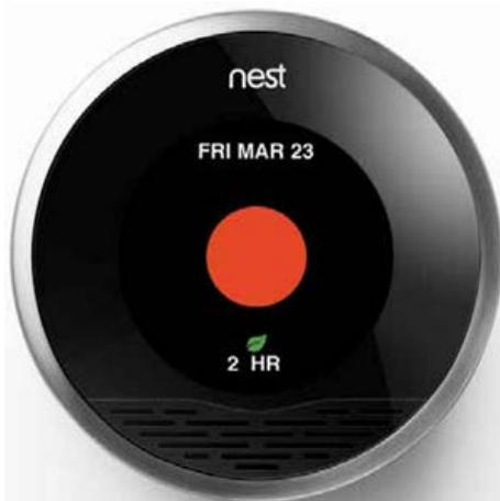
The algorithms Nest Labs has implemented based on built-in sensors enables the user to save energy with very little interaction.
